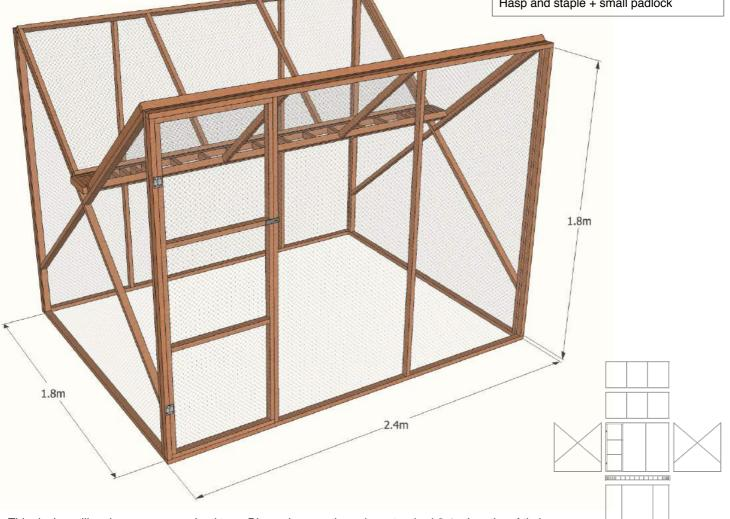
This design will make an average sized trap. Dimensions are based on standard 2.4m lengths of timber. Adjust dimensions to requirements.
